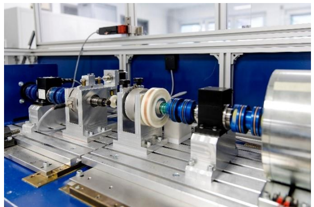
Fig. 4: In situ gear test rig developed at the LKT
