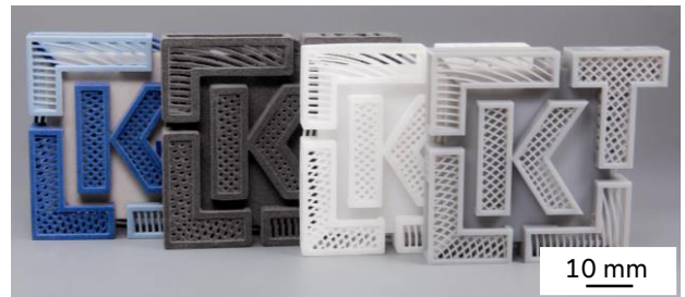
Fig. 1: Parts prepared by different AM techniques: fused filament fabrication, LPBF-P and stereolithography
