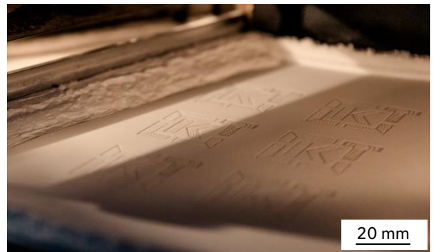
Fig. 2: Processing of polyamide 12 filled with 15 vol.-% copper beads via LPBF-P
