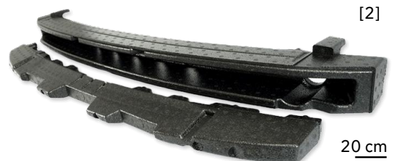
Fig. 3: Front bumper made of particle foam
