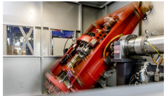
Fig. 2: Rotational molding machine at LKT
