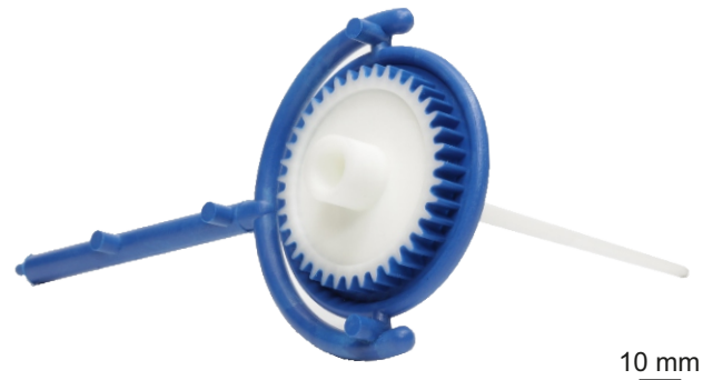
Fig. 5: Tribo-mechanically optimized 2-component gear matrix material: Polyoxymethylene (POM) inner component: POM with glass fibres outer component: POM with Polytetrafluoroethylene
