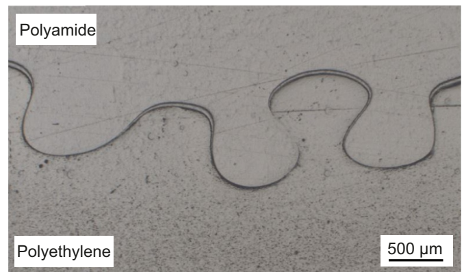
Fig. 3: Interlocking of polyethylene and polyamide within a multi-layer part
