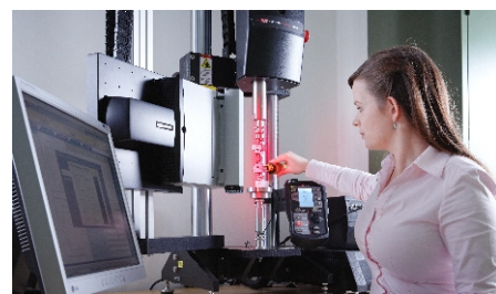
Fig. 4: Tensile testing on a universal testing machine
