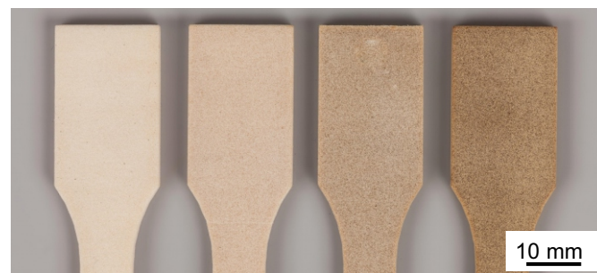
Fig. 8: Photography of PA 12 tensile bars at different aging stages for the determination of longterm properties; storage temperature: T = 140\text{ }^{\circ}\text{C} , from left to right: 72 h, 168 h, 336 h and 672 h
