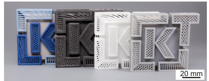
Fig. 1: Parts prepared by different additive manufacturing technologies, available at the LKT From left to right: fused deposition modeling, selective laser sintering with filled material, selective laser sintering, stereolithography
