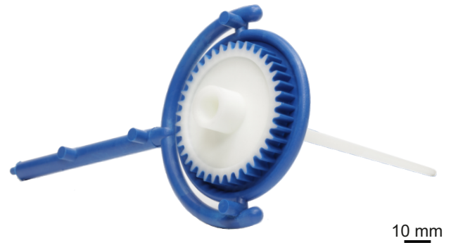
Fig. 5: Tribo-mechanically optimized 2-component gear matrix material: Polyoxymethylene (POM) inner component: POM with glass fibres outer component: POM with Polytetrafluoroethylene
