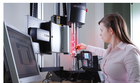
Fig. 4: Tensile testing on a universal testing machine
